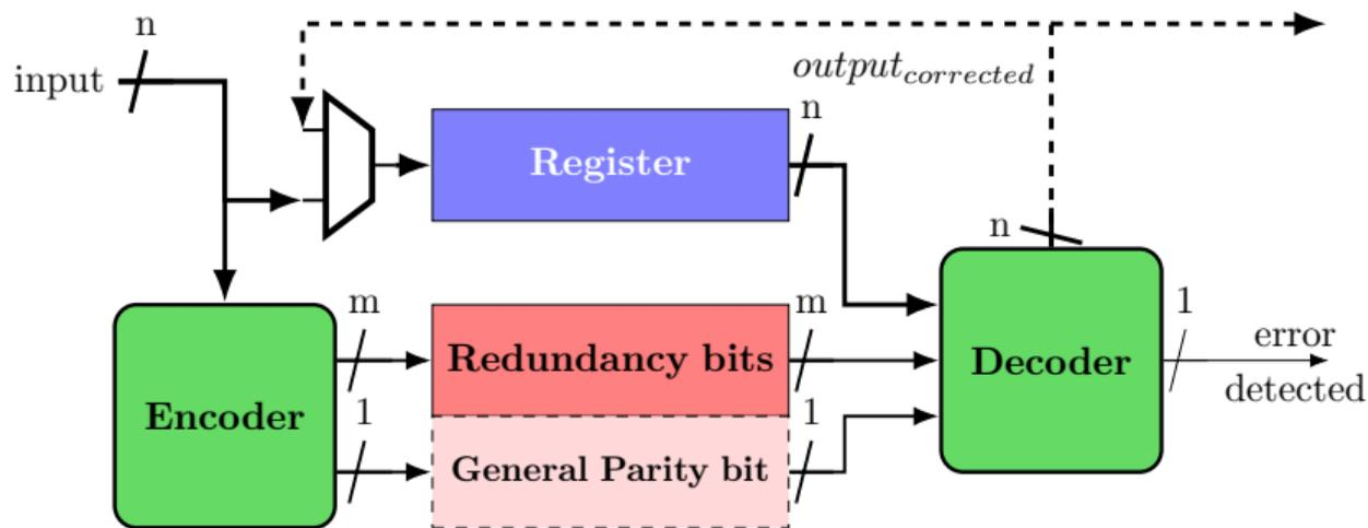
Figure 16: Implementation of a protection for one register
