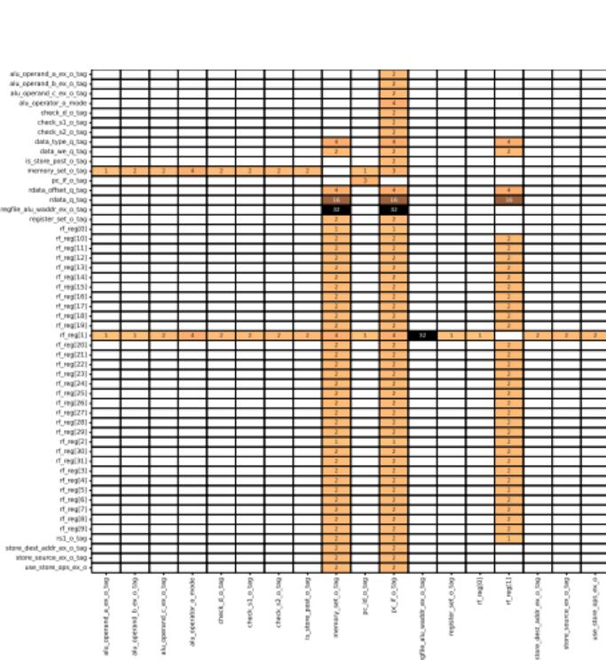
Figure 22: Unprotected version: multi-bits faults in two registers at a given clock cycle → 450 successes
