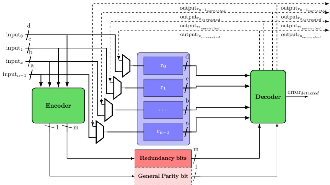
Figure 17: Implementation of a protection for multiple registers
