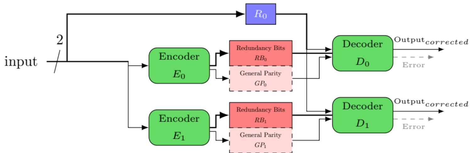
Figure 19: Implementation of a protection for one register split
